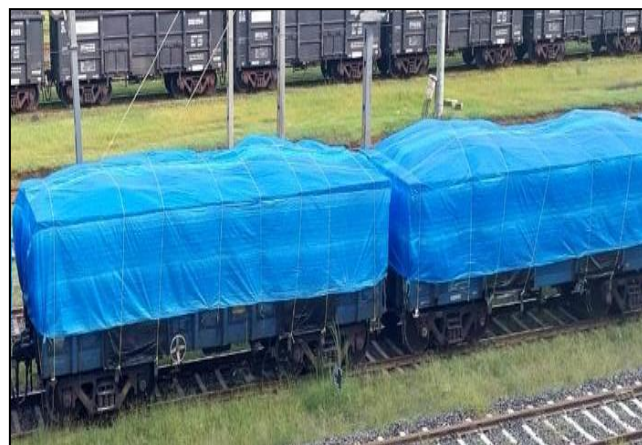
Tarpaulin covering in BOXEN rake loaded with Fly Ash
