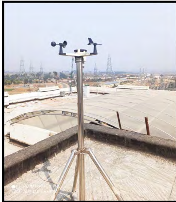
Figure 1: Weather Monitoring Station at Hostel Block
