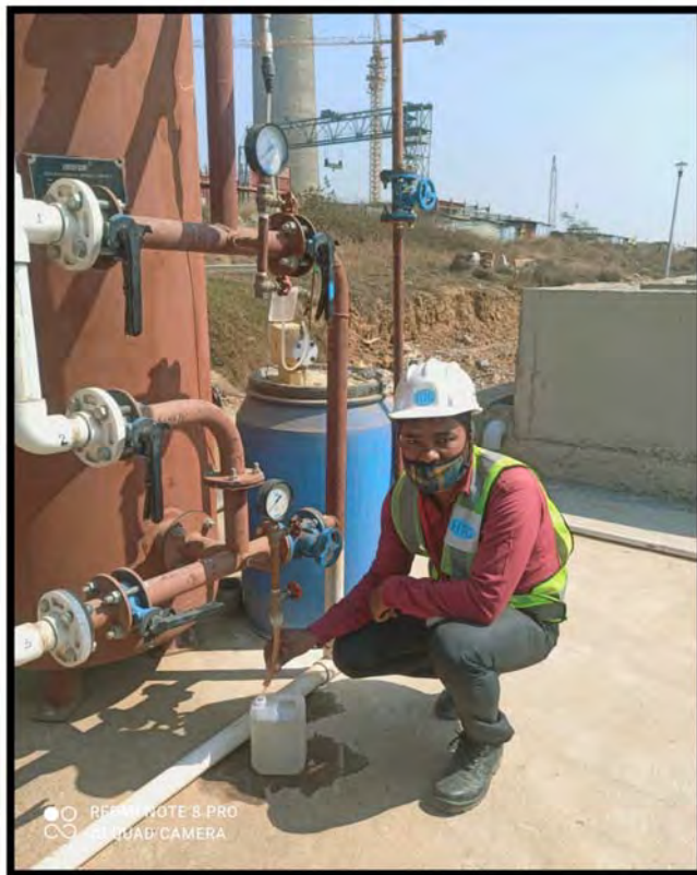
Figure 12: Water Sampling at STP Outlet township
