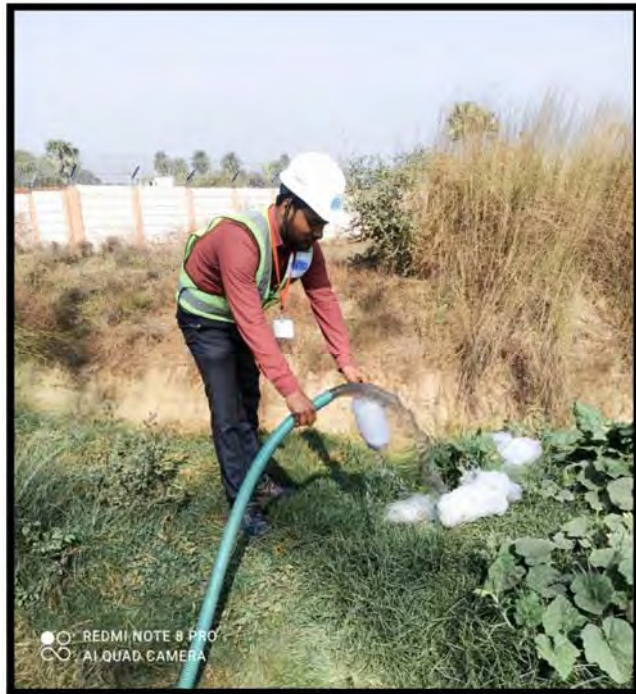
Figure 11: Water Sampling at STP Outlet plant
