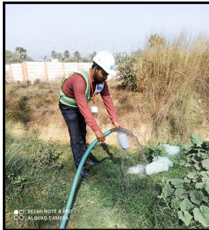
Figure 11: Water Sampling at STP Outlet plant
