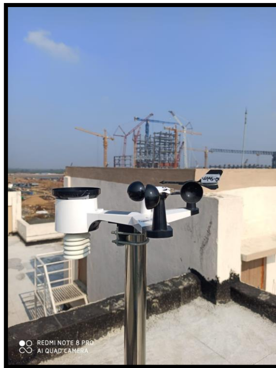
Figure 1: Weather Monitoring Station at Hostel Block
