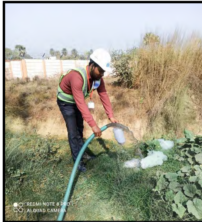
Figure 11: Water Sampling at STP Outlet plant
