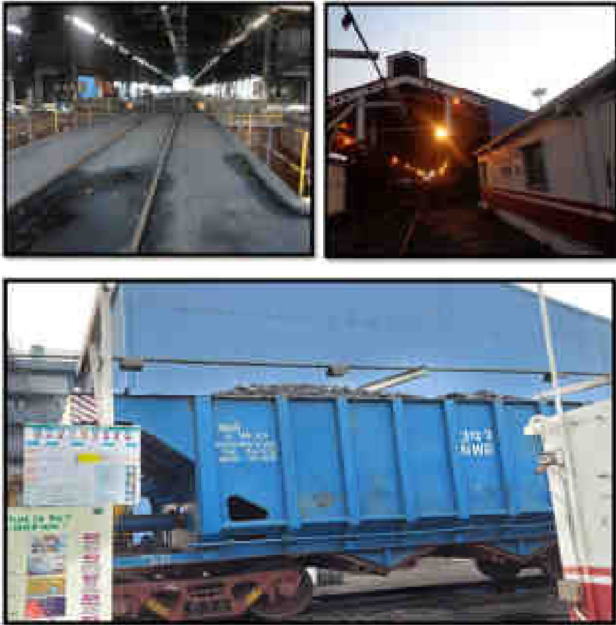
Fig 7: Pre-wetting System before entering Track Hopper for reduce fugitive dust emission
