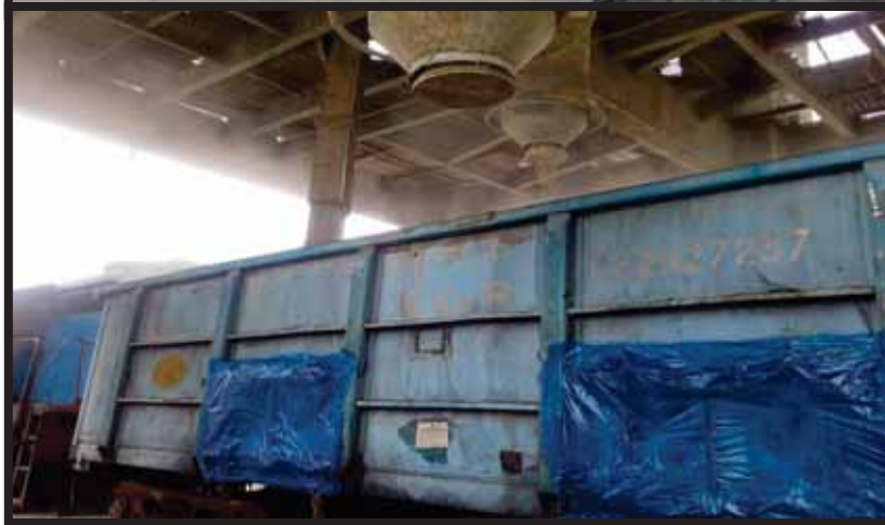
DOOR CLOSING OF RAKE FOR AVOIDING LEAKAGE/SPILLAGE DURING TRASPORTATION
