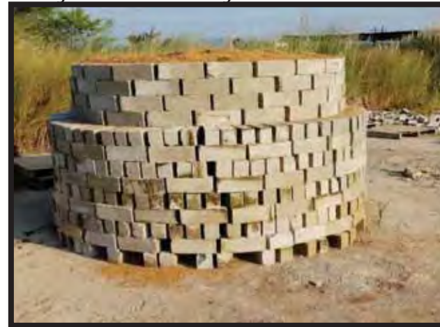
Dry Bricks heated with Rise Husk
